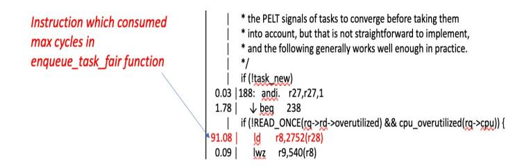
**Question**: What data type is being accessed here ? ex: basic data types like int or any struct ) **Solution**: Use data type feature in perf to solve this without manually doing perf annotate and mapping in the code
